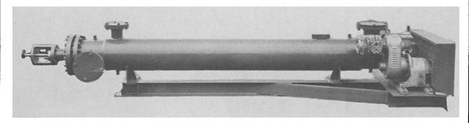
To enable you to test your crystallization problem, or your problems of viscous cooling, exothermic reactions, desublimation condensing, solvent extractions, solvent flashing or other problems involving heat transfer to highly viscous and fouling materials.
